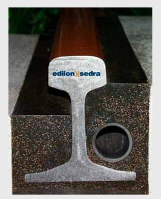
The ERS rail fastening system is characterized by continuous support of the rails, as well as by the elimination of any and all forms of small hardware components. This also means avoidance of the support-point frequencies of traditional, discrete rail fastening systems - and it enables transfer of live traffic loads more uniformly and with reduced load peaks into the supporting track substructure.
