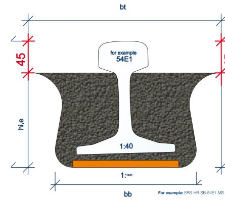
Group SB versions of ERS rail fastening systems are designed for applications in combination with steel module bridges (MB-S), or with modular steel deck plates.
