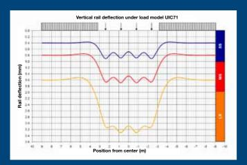
The standard designs of the ERS-HR rail fastening system are based on the UIC71 load model.
