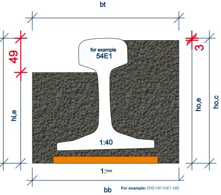
ERS rail fastening systems in Group L are designed for track areas that can also serve as level crossings or roadways for vehicles crossing the tracks, or moving along or over the tracks (e.g. for rescue and service vehicles).
