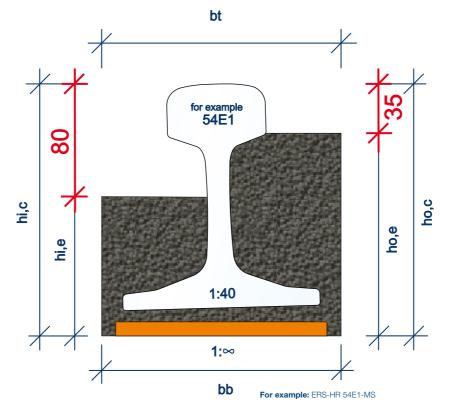
ERS rail fastening systems in Group B applications are designed for track areas that are not used by street vehicles driving along or across the tracks.
